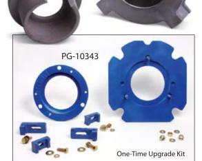
PG-10343 is required by 10D(S) shot blasters 2003 and older; and all 15D(S) models to accept the new High-Life Wheel Kit. The PG-10343 includes: Plate Adaptor; Collar; Feed-Spout Clamps and Hardware. Shown above.
